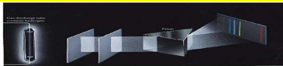
Figure 7.9 The line emission spectrum of excited hydrogen atoms. The emitted light is passed through a series of slits to produce a narrow beam of light, which is then dispersed into its component wavelengths by a prism. A photographic plate or an inverse screen detects the separate wavelengths as individual lines. Hence, the name "line spectrum" for the light emitted by a glowing gas.
